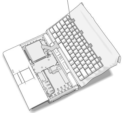
12 Gently touch the metal surface on the right side of the inside of the computer to discharge any static electric built up on your body.
